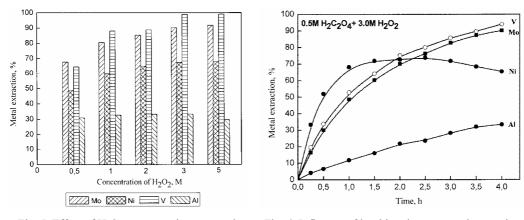
Fig. 5. Effect of  $H_2O_2$  concentration on metal leaching efficiency at 50°C in 0.5M  $H_2C_2O_4$  solution after 4 hour leaching
