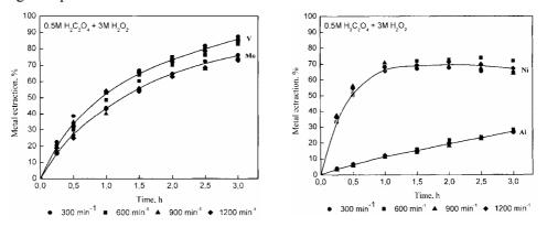
Fig. 4. Effect of stirring speed on metal extraction as a function of time at  $50^{\circ}$ C in solution containing  $H_2C_2O_2$  and  $H_2O_2$  after 3 hour leaching
