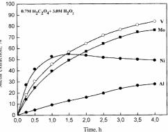
Fig. 7. Effect of H<sub>2</sub>C<sub>2</sub>O<sub>4</sub> concentration on metal leaching efficiency at 50°C in 3.0 M H<sub>2</sub>O<sub>2</sub> solution after 4 hour leaching
